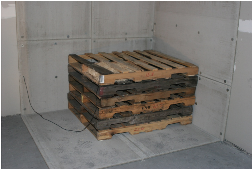
Figure 2. Pallets and Excelsior Ignition Source Used as a Fuel Source
