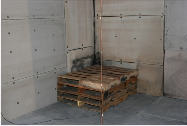
Figure 3. Fuel and Excelsior Source for Slow (left) and Fast (right) Ignition Scenarios
