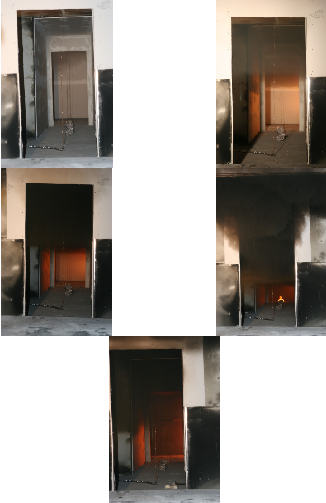
Figure 5. Example Fire Progression from Test CRA 1
