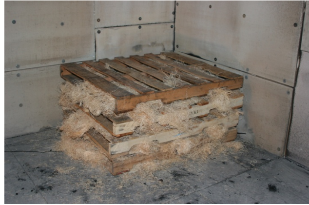
Figure 3. Fuel and Excelsior Source for Slow (left) and Fast (right) Ignition Scenarios
