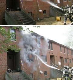
These photos show the rapid reduction in heat release rate (fire size) from the application of water to the island to film. The segment provides an from an exterior position from of the "burned side" of the building, when no other vents to the exterior are open.
