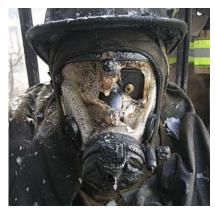
Opening the door provided additional air to a smoldering living-room fire and caused the fire to increase in burning rate and flames to extend out the doorway, resulting in high temperatures and heat flows that melted a hole in the mask. Pressure sensor (brass fitting that was mounted on the face of the headform) is visible through the hole in the lens. Credit: NIST
