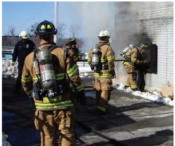
Figure 23: Supplemental Suppression Applied for Room and Contents Tests
